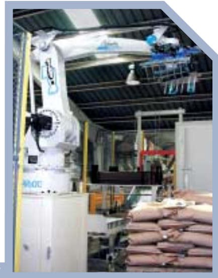
1. Mendota's new robotic palletizer and automated shrink wrapping capability provide labor efficiency and improved employee safety benefits.
